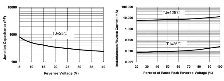
**Fig.1-Typical Junction Capacitance**
