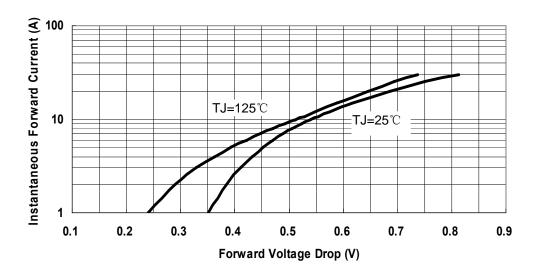
Fig.3-Typical Instantaneous Forward Voltage Characteristics
