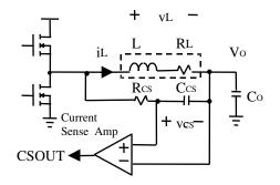
Figure 4: Inductor Current Sensing and Current Sense Amplifier
