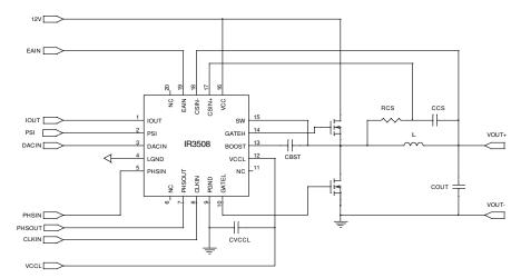
Figure 1 Application Circuit
