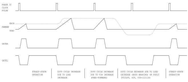
Figure 3: PWM Operating Waveforms
