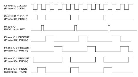
Figure 2: Four Phase Oscillator Waveforms
