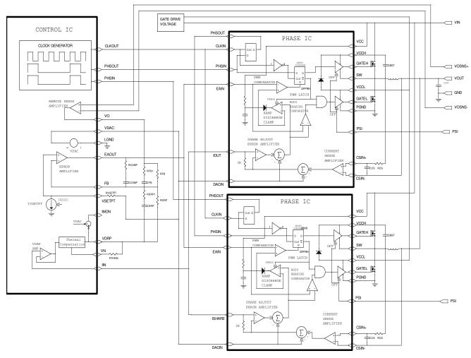
Figure 1: PWM Block Diagram
