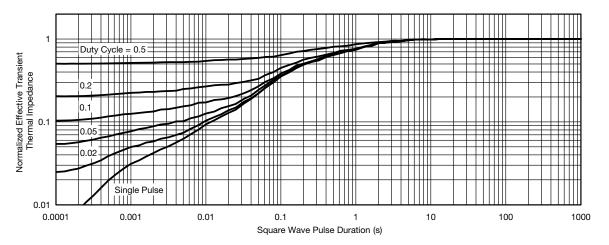
Normalized Thermal Transient Impedance, Junction-to-Foot
