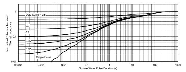
Normalized Thermal Transient Impedance, Junction-to-Ambient
