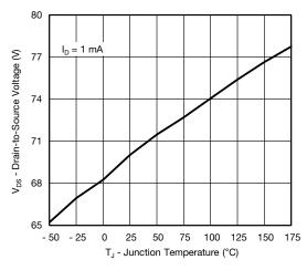
Drain Source Breakdown vs. Junction Temperature
