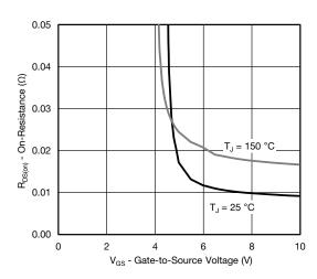
On-Resistance vs. Gate-to-Source Voltage
