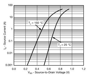
Source Drain Diode Forward Voltage
