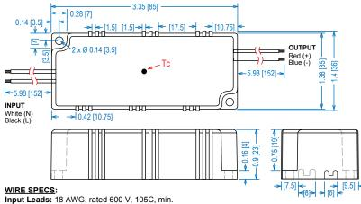
Input Leads: 18 AWG, rated 600 V, 105C, min. Output Leads: 18 AWG, rated 300 V, 105C, min. All wires are stranded with solder dipped ends.
