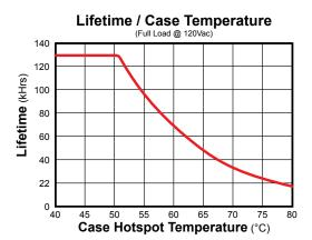
Note: The area under the life-temperature curve represents where the driver has highly reliable operation within specification. Driver performance may drift out of published specifications as the hours of operation exceed the curve at a given temperature. Higher operating temperatures increase the chances of a failure to function. Other electrical, mechanical and environmental factors affect driver lifetime but are not represented in this calculation.
