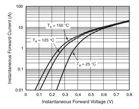
Fig. 3 - Typical Instantaneous Forward Characteristics Per Diode
